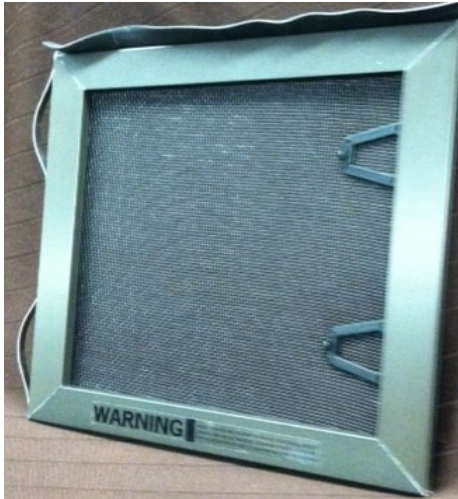
SIDE-LOAD SCREEN (5/16 extruded stock) slide-on springs & plastic tabs on height optional rubber bug flap on top with or without BUMP on back
